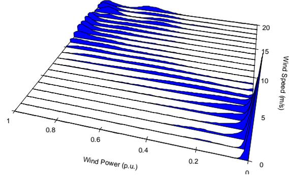
Fig. 1. Example of tacked conditional plot for wind power (axis to the left) and forecasted wind speed (axis to the right).
