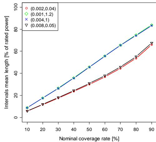
Fig. 10. Sharpness diagram for different kernel bandwidths  $(h_{Power}; h_{WindSpeed})$ .
