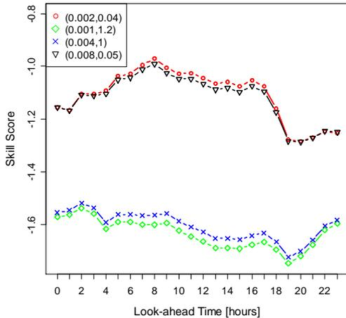
Fig. 11. Skill score diagram for different kernel bandwidths ( $h_{Power}, h_{WindSpeed}$ ).
