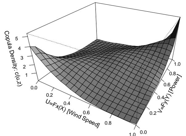
Fig. 2. Bivariate copula density function of forecasted wind speed and measured wind power.
