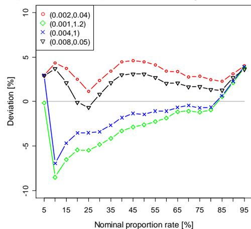
Fig. 9. Calibration diagram for different kernel bandwidths  $(h_{Power}; h_{WindSpeed})$ .
